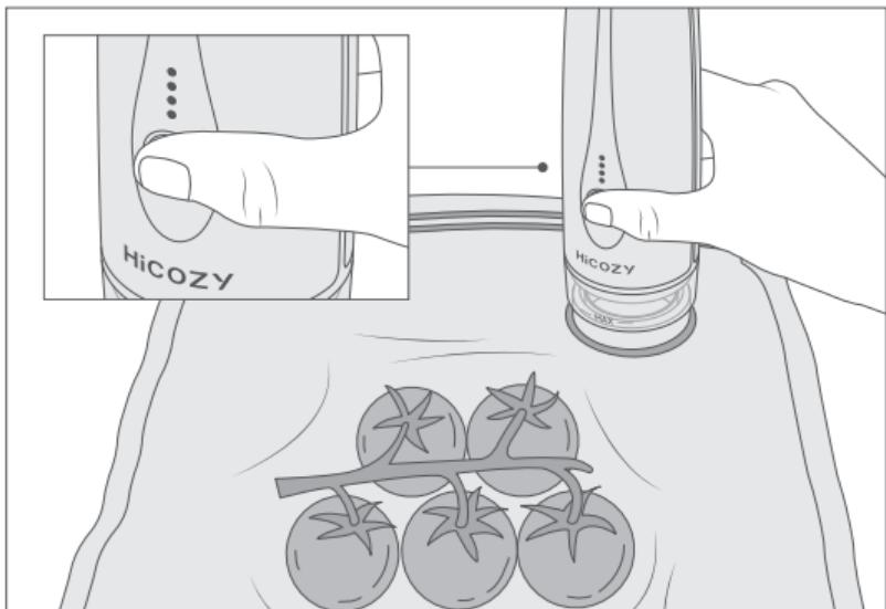
4. When the bag is sufficiently vacuumed, the machine will automatically stop. When it stops, the operation button indicator will flash to signify completion before turning off.
