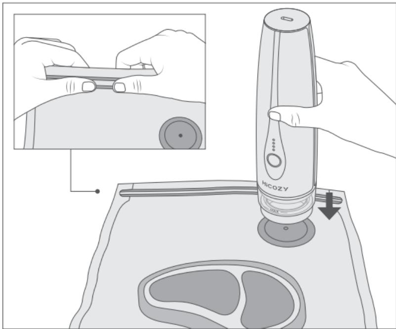
2. Press and hold the button for 2 seconds to turn on the machine. The power indicators and operation button will light up and the machine will start to vacuum and drain water.
