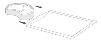
Step 2: Put the unsealed end under the 3 markers in the vacuum channel and close the cover.
