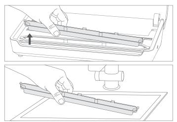
If the seal rings are deformed or fall, pull the seal rings out of the slot. Then, replace the old rings with new seal rings by firmly pressing them into the slots. Ensure they are securely inserted.
