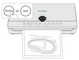
Step 5: After the suction power is set, press the Dry or Moist Button according to the food's moisture level. The machine will automatically start vacuuming and sealing the food, it will beep twice when the seal is complete.
