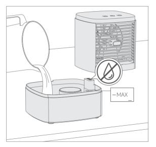
**Note:** Do not add ice to the atomizer. Do not allow water to contact any of the electronics.
