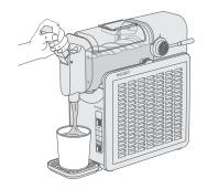
7. Clean the machine immediately after dispensing the frozen drink to make cleaning easier. (For detailed cleaning instructions, refer to the "Cleaning & Maintenance" section of this manual.)
