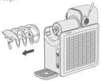
3. Scrub the evaporator and its sealing ring with a clean, soft towel. Do not disassemble or pull on the seal ring, as this may cause deformation and lead to water leakage.
