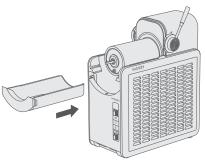
3. Install the auger and ensure it is properly aligned with its designated hole during installation.
