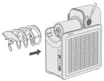
4. Install the vessel by inserting it between the water pan and the auger.
