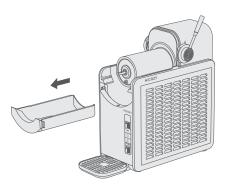
5. Wipe down the area underneath the evaporator with a sanitized or warm, damp cloth.
