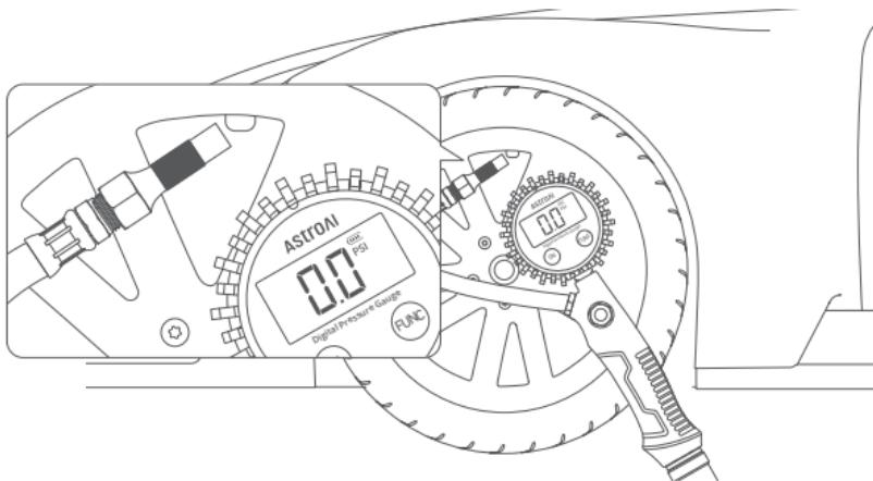
3. Press the LCD Button to turn on the screen. Press it again to choose the desired unit. 4 options: PSI, Bar, kPa, kg/cm<sup>2</sup>.
