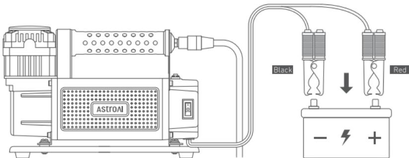
5. Pull the airflow valve downwards and switch the Power Button of the air compressor to the "I" side to start the air compressor.
