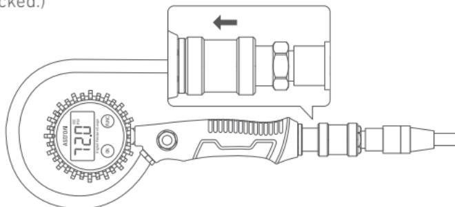
7. When the pressure reaches the manufacturer-recommended level, press the Power Button to the "0" side and remove the air hose from the tire stem.
